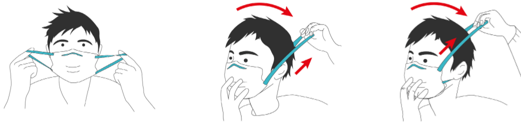
Figure E.4: Placement of the head harness
